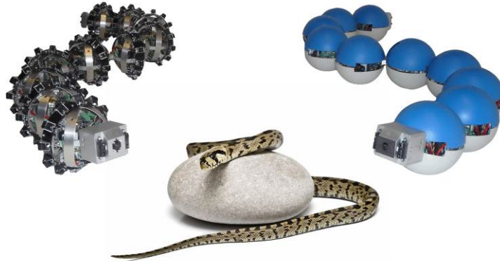
Figure 2: Examples of snake robots (the NTNU/SINTEF snake robots Wheeko, left, and Kulko, right) and a biological snake.
