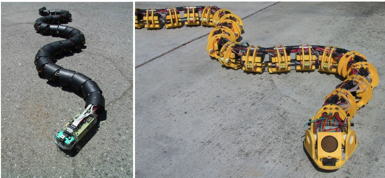
Figure 13: The snake robots S5 4 (left) and S7 5 (right) developed by Dr. Gavin Miller. The robots have passive wheels on their underside.
