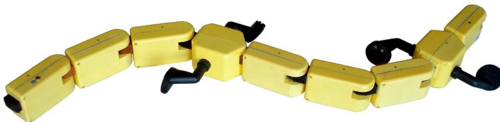
Figure 20: A salamander-like snake robot 11 developed at Ecole Polytechnique Fédérale de Lausanne (EPFL). The robot uses motorised legs to propel itself forward and can operate under water.
