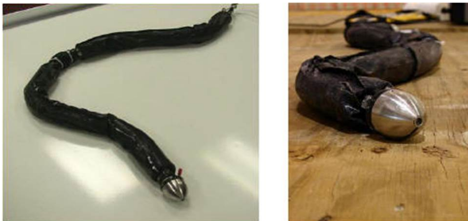
Figure 19: A snake robot with a skin drive 10 propulsion system developed at Carnegie Mellon University. A motor drives the outer skin backwards along the snake body in order to propel the robot forward.
