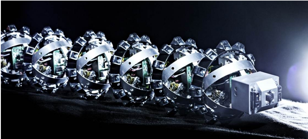
Figure 14: The snake robot Wheeko 6 developed by SINTEF and NTNU (the Norwegian University of Science and Technology). The robot consists of many 2-DOF joint modules covered by passive wheels.
