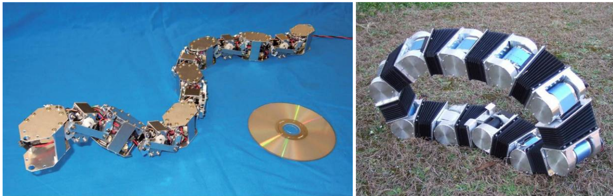
Figure 16: Two snake robots developed at Tokyo Institute of Technology. The robot on the left [10] demonstrates a miniature joint mechanism, while the robot on the right [11] can perform so-called loop forming motion.
