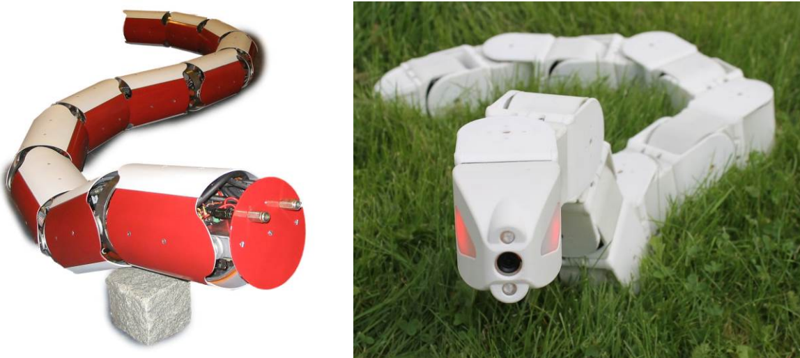
Figure 17: The snake robots Anna Konda 8 (left) and Mamba 9 (right) developed by SINTEF and NTNU. Anna Konda is a water hydraulic snake robot developed to demonstrate firefighting applications. Mamba is watertight and can measure external contact forces using a strain gauge based force sensor system.
