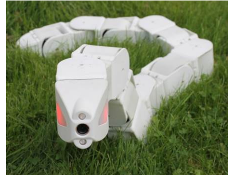
The NTNU/SINTEF snake robot "Mamba".
