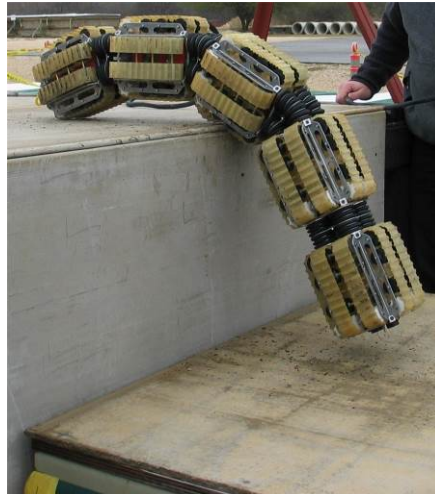
Figure 18: The OmniTread snake robot [14] developed at the University of Michigan. The robot has pneumatic joints and is covered by motorised tracks.
