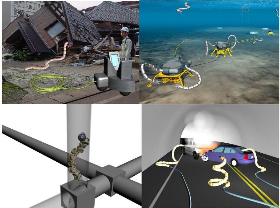
Terrestrial snake robot applications: search and rescue (top left), subsea operations (top right), inspection and maintenance (bottom left), and fire-fighting (bottom right).
